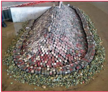
Figure 16: Model of a breakwater
