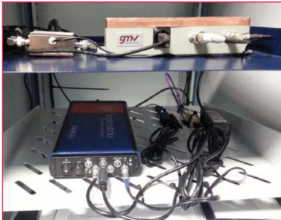
Figure 3: GNSS Receiver and GPS L1 Interference Detector
