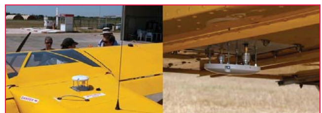
Figure 3: Antennas on the top (left) and on the bottom (right) side of the plane
