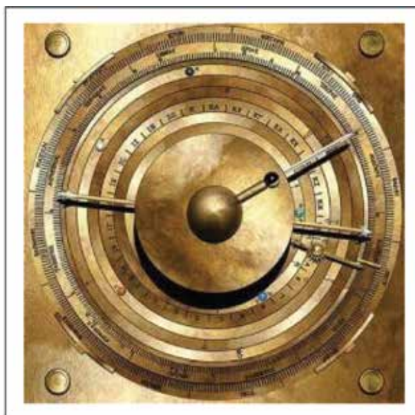
Figure 6: Virtual Reconstruction of the Front Dial. As with Wright's physical reconstruction, the two outer dials on this reconstruction of the Mechanism are the zodiacal and calendrical scales [Freeth et al., 2021]. None of inner scales are thought to serve as a sliding nonius which might have enhanced the precision with which the zodiacal scale may be read.
