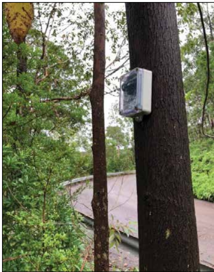
Figure 1: A prototype sensor has been installed on lower tree trunk to measure the displacement angles and the collected data will send to our Spatial Big Database for data analysis
