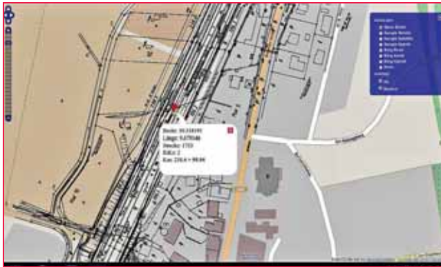
Figure 6: Tablet with Position Marker related to the track infrastructure
