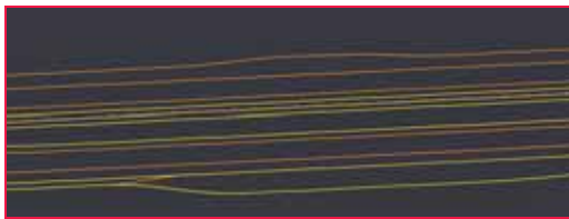
Figure 10: Example of the vector data from SD card visualized in the German rail-network, showing track rails (yellow), the stationary rails (orange) and the routing (pink points) – always with the information of the explicit track number, chainage and coordinates
