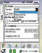
Static, Fast Static and Stop&Go surveying
