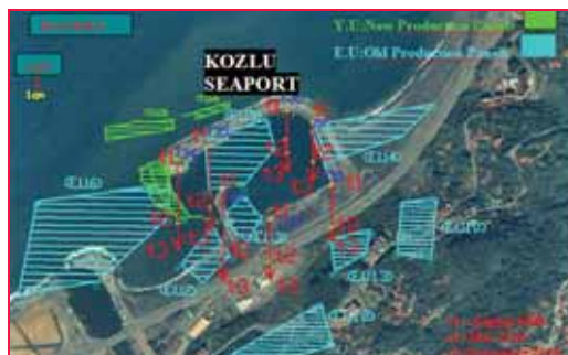
Figure 5: Vertical displacement vectors obtained from the precise leveling measurements in Kozlu Seaport.
