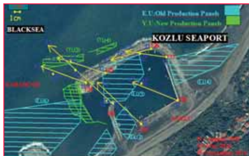
Figure 4: Horizontal displacement vectors obtained from GPS measurements in Kozlu Seaport.
