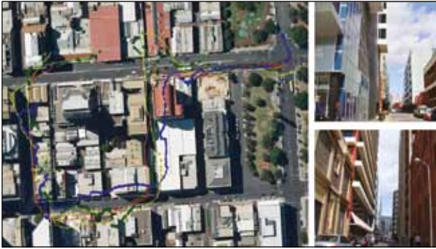
Figure 4. Kinematic test results of HSGPS receivers in an urban canyon environment (iPhone 3GS – red cross; iPhone 4 – yellow diamond; iPaq 914c – blue dot; N95 – green square; real ground track – white; start point – red star; end point – green triangle)
