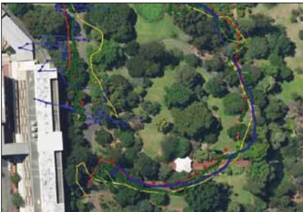
Figure 6. Kinematic test results of mobile phones in a forested area (symbols are the same as in Fig. 4, however there is no real ground track to provide "groundtruth")
