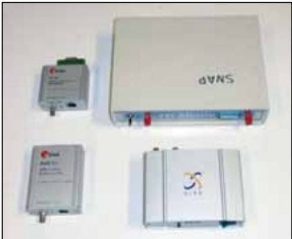
Figure 1a. HSGPS receivers used in the tests (from left to right, top to bottom: ublox LEA-4P, Navman Jupiter 32, ublox EVK-5H and SiRF GSCI-5000)
