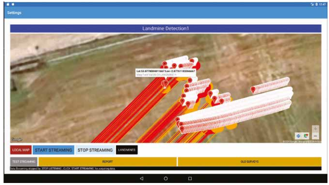
FIGURE 21. Landmine locations, until the current scanned point in the route, shown by user during data streaming while Maggy is still in operation.
