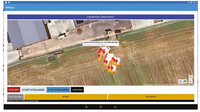
FIGURE 23. Landmine locations, with "very high" (red) and "high" (orange) MF, shown by the user.
