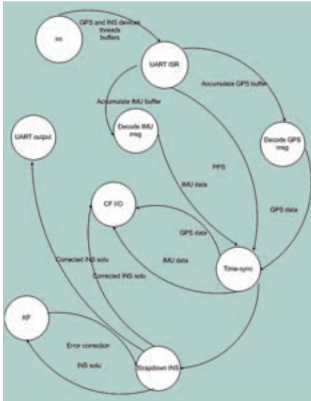
Figure 3. Operation diagram of the embedded software
