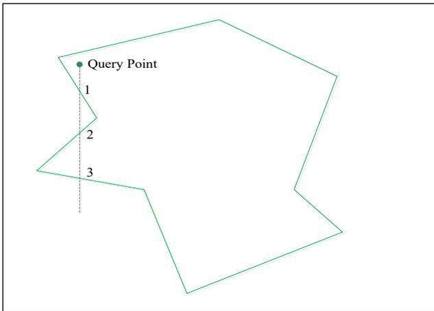
Figure 9. Point in polygon test (point inside the polygon).
