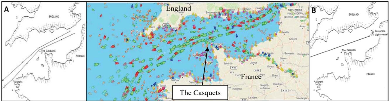
Figure 3: Middle picture shows shipping in Dover Straits. Picture A (left) shows the traditional in and outward bound of shipping pattern in Dover Straits. Picture B (right) shows in and outward bound of shipping pattern using radio navigation. Source: Hooff, (1982); www.marinevesseltraffic.com (2016)
