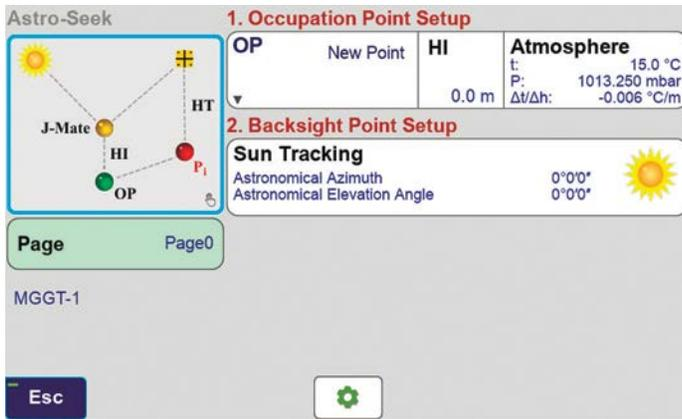
We have added a new innovative feature to the J-Mate that it can automatically calibrate itself via its automatic Sun or other astronomical objects-Seeking feature.
