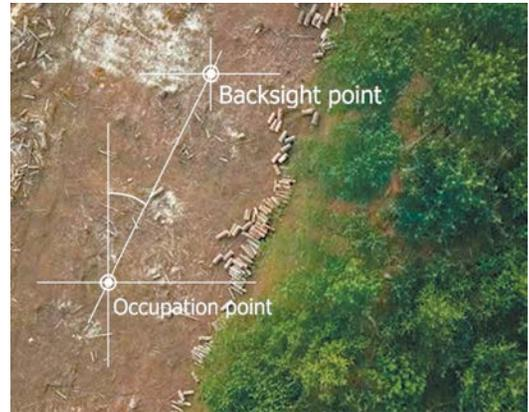
This screen appears which guides you to determine the accurate positions of the Occupation Point and the Backsight Point, to establish an azimuth and calibrate the J-Mate angular encoders.
