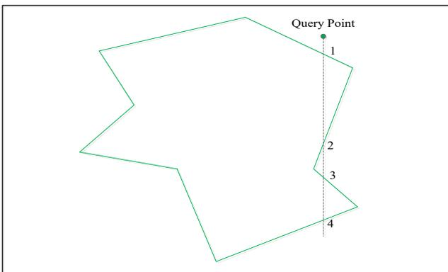
Figure 10. Point in polygon test (point outside the polygon).
