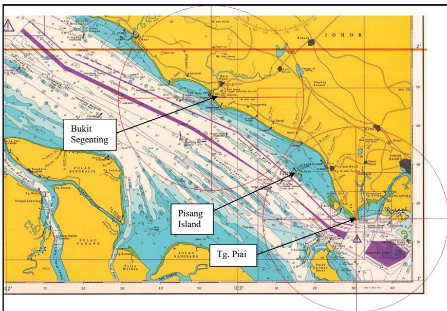
Figure 6: The existing VTS radar Coverage
