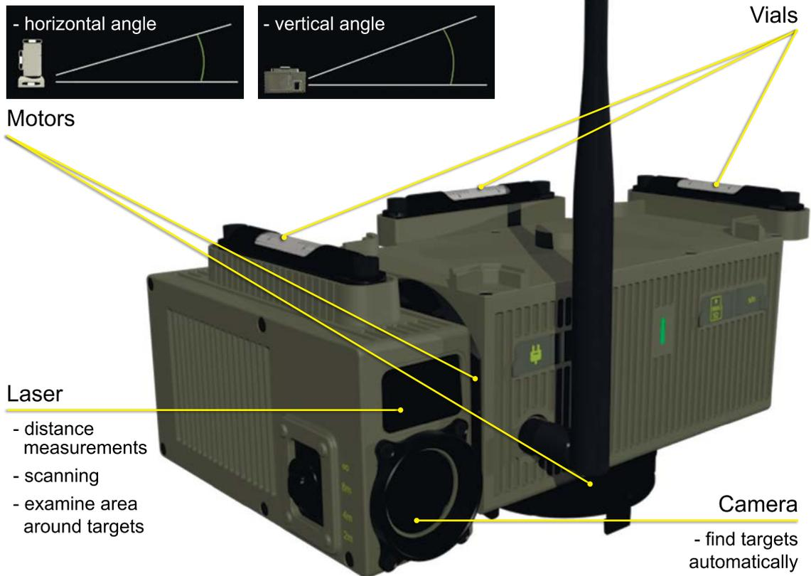
Similar to using conventional total stations, to use the J-Mate you need first to establish its accurate position and calibrate its vertical and horizontal encoders. Then proceed to shoot the unknown points. This is similar to using any total station, but we have improved and automated the process.
