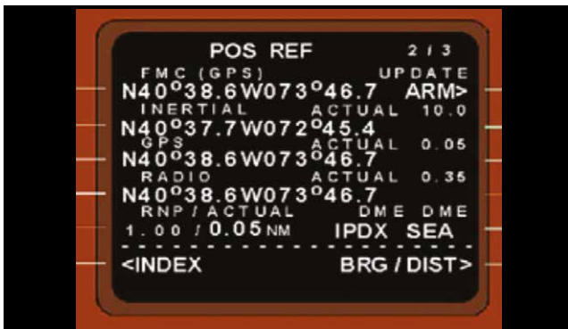
Figure F3: The navigation system in the representative FMS. Based on the available navigation aids and the required performances, different combinations of sensors can be used. It is visible that the flight computer is taking only the GPS position due to its high accuracy (0.05 with unit in NM), for the navigation and guidance. The accuracy is indicated by the ACTUAL value. The logics in the FMS and the pilot choices overwrite the selection and combination of sensors.
