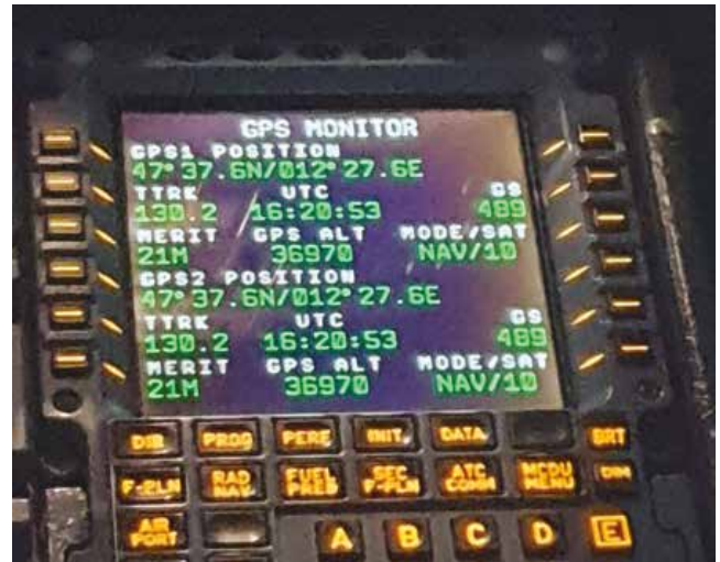
Figure F4: The flight computer that computes the real-time PVT of the space vehicles/aircraft based on GPS satellites. The figure of merit shows confidence of 21 meters accuracy, and the used number of satellites is 10. When the figure of merit value is inflated to compute the protection level, 0.1 NM is easily attainable. The approach procedure of LNAV/VNAV (see Figure F5) with 0.3 NM can be flown only based on GPS positioning.
