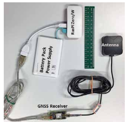
Figure 5: A plug-and-play type of L-CHAPS to log GNSS data for post-processing RTK
