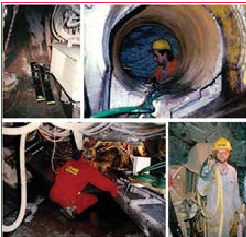
Figure 6: GPR 100 MHz antennas (top left), Manhole with fibre optics (top right), engineers passing GPR equipment through a manhole (bottom left) and carrying protection tubes for the vulnerable fibre optics (bottom right). Photos: E Meier, U. Sambeth.
