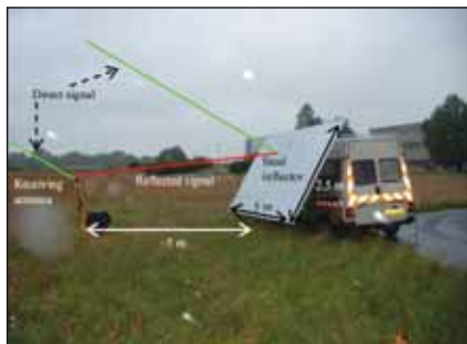
Fig. 2 Diagram showing the geometry of the LCPC test datasets
