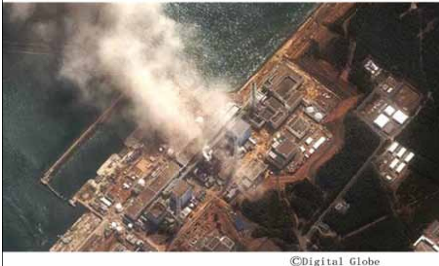
Fig.3 Accident of Fukushima Nuclear Power Plants with Hydrogen Gas Explosion
