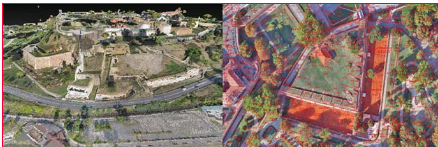
Figure 6: Point cloud (left) and ortho-photo map by using UAV technology overlapped with cadastral data for the location Kalemegdan fortress in Belgrade
