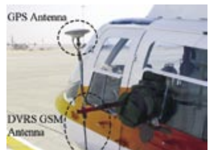
Figure 2. System installation for the helicopter test
