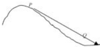
Fig. 1 A receiver at point Q receives the light signal with frequency f emitted by an emitter at P, where P and Q are located on the Earth's surface
