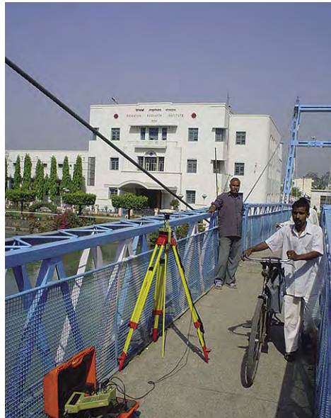
Figure 1 Observation Station on the Cable-Stayed Bridge [on Ganga Canal near Irrigation Research Institute (IRI) Roorkee].
