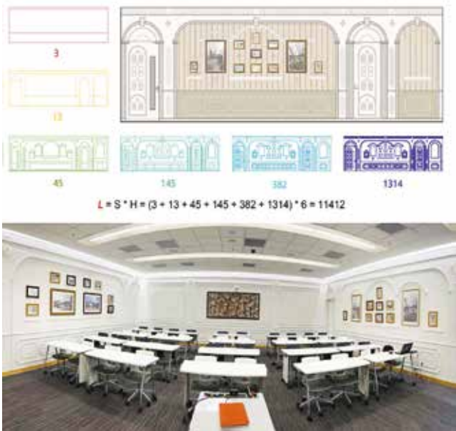
Fig. 7. Classroom W1-233 before and after renovation. Top: original room with undifferentiated long wall. Middle: declared skeleton (six levels of scale, 2–6 ratio). Bottom: realised renovation — paneling, mouldings, framed artworks — expressing the skeleton. L-score rose by an order of magnitude; mirror-of-the-self preference favoured the renovated condition (Table 1).
