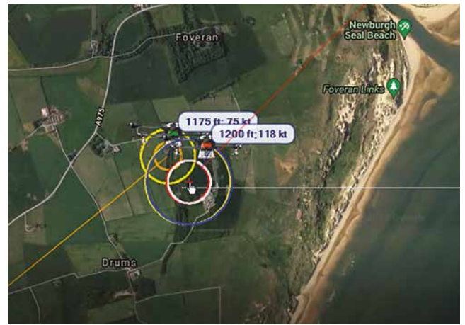
Fig. 14. Self manoeuvring using the simulated and real flight data: Red ICTZone and heading and yellow PCTZone within the original path; white ICTZone and heading and blue PCTZone within the manoeuvring trajectory. (For interpretation of the references to colour in this figure legend, the reader is referred to the web version of this article.)
