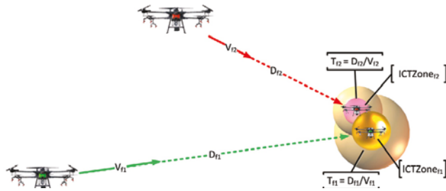
Fig. 10. Estimation-based predictive display: Early warning for a collision risk concerning an impending crossing point (impending crossing within I_{crZ} ) with two flights that have different velocities and are flying at similar altitudes. V , D and T correspond to "velocity", "distance" and "time to reach the crossing point" respectively.
