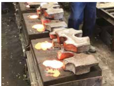
Figure 11: Sand blocks with molten alloy poured.
