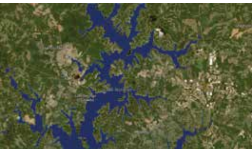
Flooding around Lake Norman in North Carolina caused by Hurricane Helene on October 7, 2024. The blue areas of the image are the Prithvi foundation model demo's prediction of the extent of the flooding. NASA
