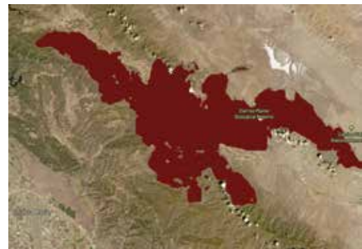
Prithvi's demo prediction of burn scars from the Gifford Fire, which occurred northwest of Los Angeles on August 17, 2025. When deployed aboard an Earth-observing satellite, foundation models can perform advanced analyses before the data even reaches the ground. NASA
