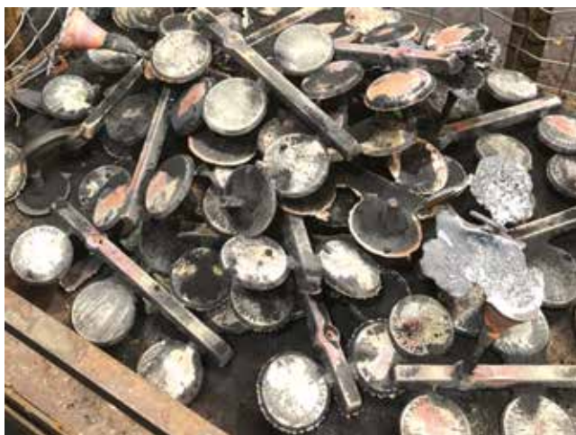
Figure 12: Stack of freshly cast type 16 PSMs ready for final staging.
