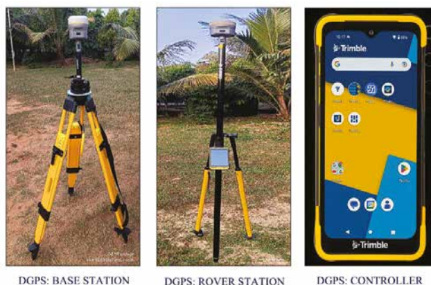
Fig. 2. Differential geographic positioning system (Base, Rover Station & Controller)
