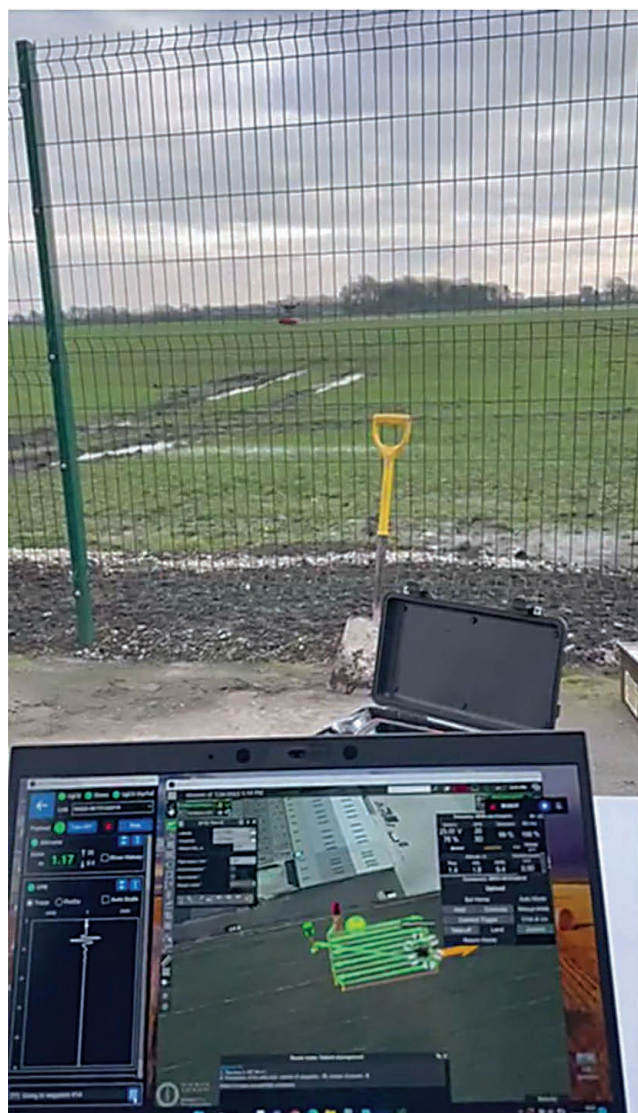
FIGURE 6. Autonomous mission monitoring in the UCLan landmine field. The drone (Fig. 5) is flying with an altitude of 1 m at a 1 m/s flight speed.
