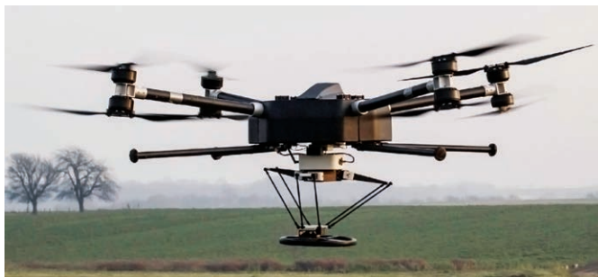
FIGURE 1. MANTA Mine Kafon 1 : GPR and metal detectors.
