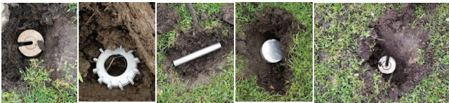
FIGURE 9. Examples for the plastic and metal landmines in different depths in the UCLan landmine field (Fig. 8).
