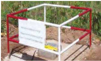
Figure 3: Pillar of the second order RCGN (Republic of Cameroon Geodetic Network) (Carmel, 2012)
