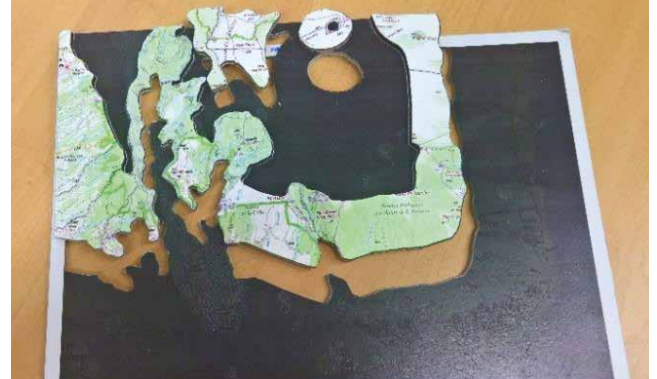
Figure 10. Separation of odd and even layers.
