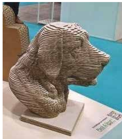
Figure 2. Stratoconception® from CIRTES to make a 3D dog head with layers of cardboard.
