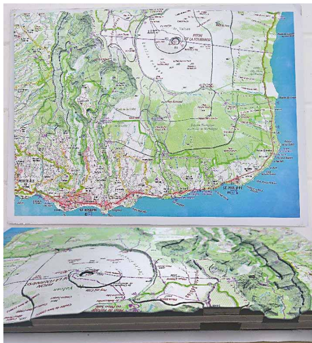
Figure 12. Relief map after the mounting, with the layers of support stacking up.
