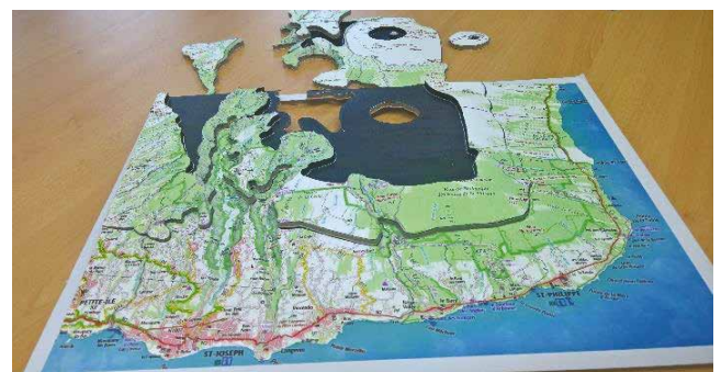
Figure 11. Mounting of odd and even layers stacking to create the relief map without height limitation.
