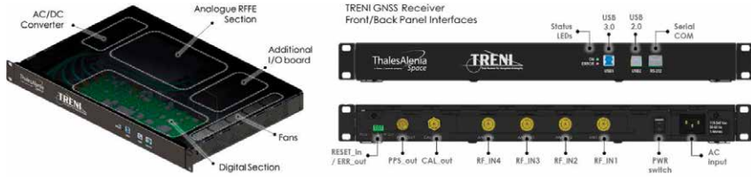
Figure 7: TRENi DFMC GNSS Receiver architecture layout (left) and interfaces (right)
