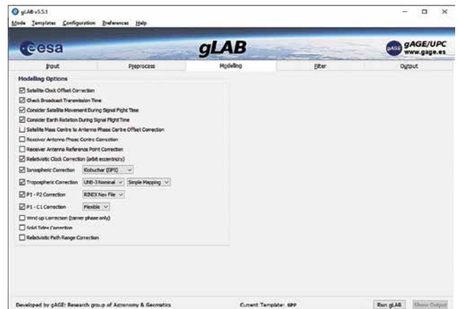
Figure 3. Modelling tab of gLAB GUI with default options selected for the SPS.
