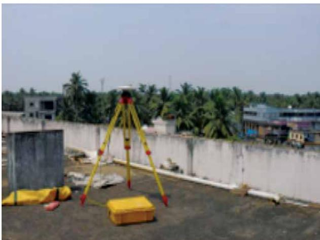
Fig 3 : Geodetic GPS receiver – Base station
