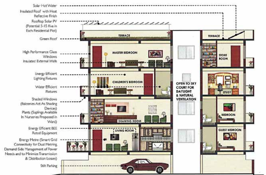
Fig. 15: Typical Section of Proposed Residential Building in Compliance with Energy Conservation Building Code Source: DUAC/Amit Ghoshal (2014), Punjabi Bagh Project, DUAC, New Delhi
