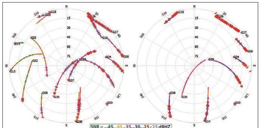
Figure 2. Skyplots showing the tracked GPS satellites of the Google Pixel 5 on L1 (left) and L5 (right) with coloured visualisation of the Signal to Noise Ratio (SNR).
