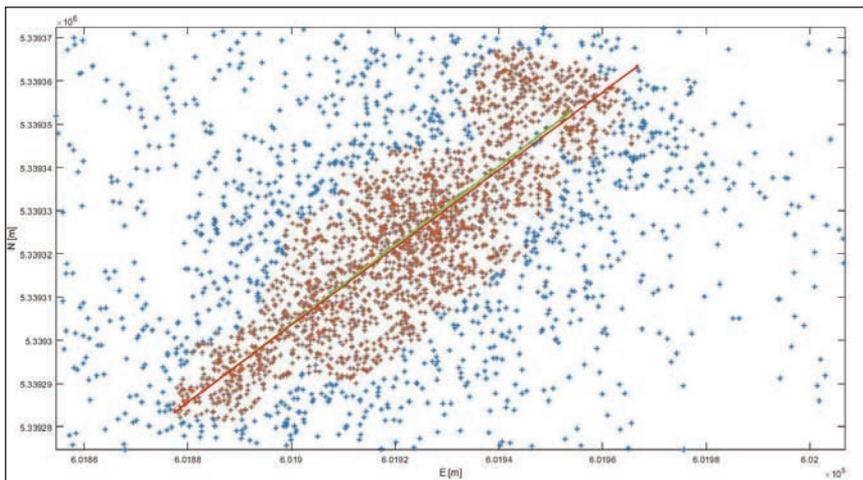
Figure 6. Adjusted line of the point cloud along the straight route. The distance calculated from the known coordinates is shown in green. The distance calculated with the help of the neighbourhood analysis from the points is shown in red. The red points have been included in the calculation of the adjusted line (Source: Retscher and Weigert (2022)).
