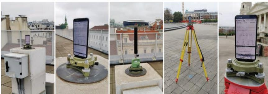
Figure 1. Smartphone und reference receiver SP80 on two neighbouring measuring pillars on the roof of the EI building of TU Wien and mobile measuring set-up on Karlsplatz.
