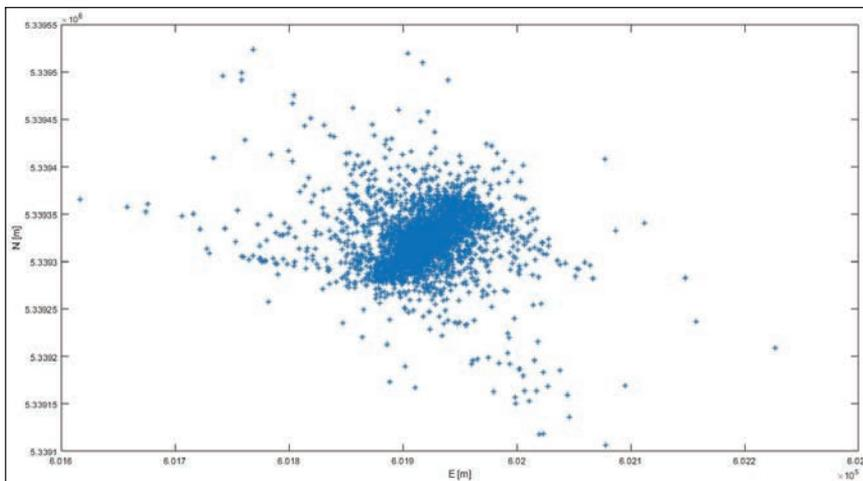
Figure 5. Point cloud with SPP solutions along the route to be investigated. The point cloud includes solutions for the round trip, as well as for all four GNSS.
