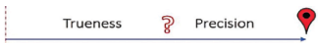
Figure 8 – A single position measurement at a point has 2 unknowns : The weight of deterministic (Trueness) errors compared to those that are not (Precision)
