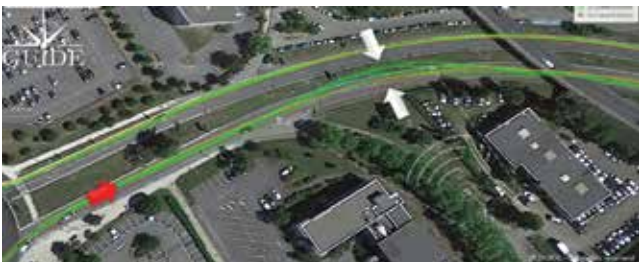
Figure 6 – Effect of unidentified temporary interference on signals for GNSS receiver
