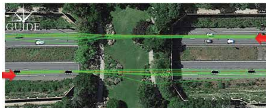
Figure 3 – Effect of alteration of GNSS signals on receivers passing under a bridge
