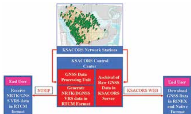
Figure 2. The KSACORS Control Unit Structure.
