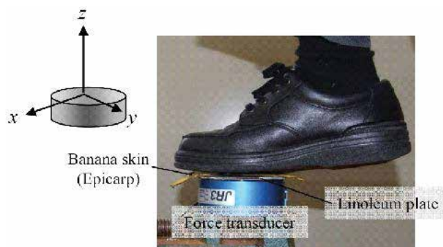
Figure 4: Experimental set-up to measure the friction coefficient under banana skin and the coordinate system used (Mabuchi et al., 2012).
