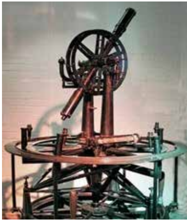
Image 3 – A "Great Theodolite" of the era of the Great Trigonometric Survey. Courtesy of B. Nagarajan, Geodetic & Research Branch Museum, Survey of India
