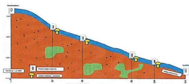
Figure 3. River level profile with GNSS points and level benchmarks
