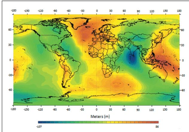
Figure 1: EGM2008 geoid heights interpolation on 2.5x2.5 minutes grid. (Source: [http://earth-info.nga.mil/GandG/wgs84/gravitymod/egm2008/egm08\\_wgs84.html](http://earth-info.nga.mil/GandG/wgs84/gravitymod/egm2008/egm08_wgs84.html))
