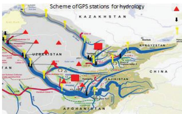
Figure 2. Scheme of GNSS network for hydrology
