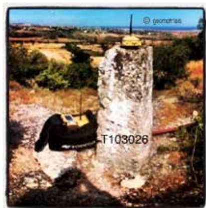
Figure 3: A common benchmark of the State's network between the two versions of the old datum.
