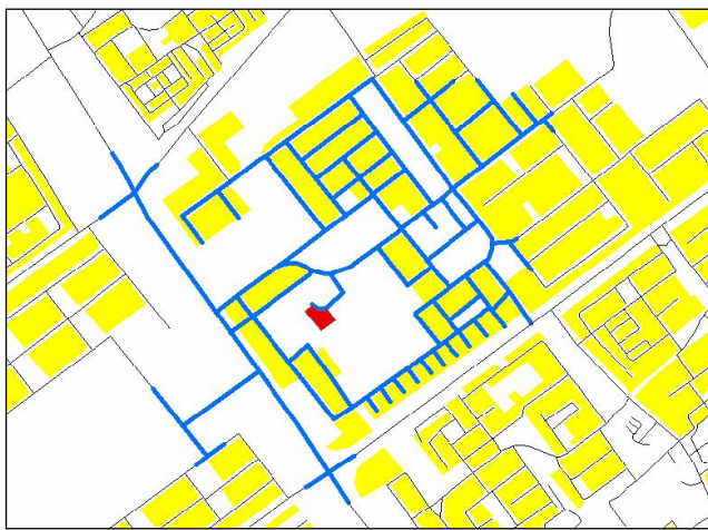
Figure 5 – Maximum 800 m walkability – Only the Residences (in Yellow) with Blue Road in front of them are in the catchment area of the Dispensary (in Red).
