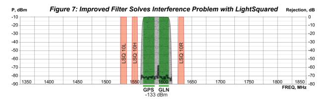
This improved filter design should make it clear that LightSquared can coexist with GNSS. Once we understand that, we can also understand that high-precision GNSS receivers can benefit from LightSquared. We can use LightSquared for RTK communication (the land-based signals that augment signals from GPS satellites and provide more precise positional data). We desperately need better RTK communication, and LightSquared's network can provide it.
