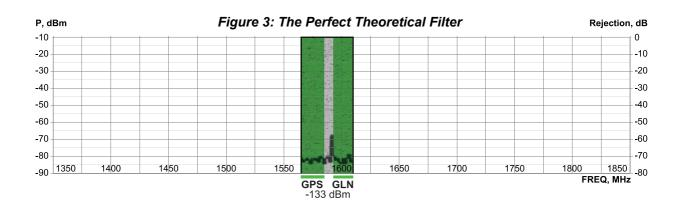
Unfortunately, it is not technically possible to build such a perfect filter. Our challenge is to build the best filter that keeps the GNSS signals intact and blocks unwanted signals as much as possible. In other words, make the side slopes, or skirts, of a filter as steep as possible. How difficult it is to build such a filter? How much would it cost?
