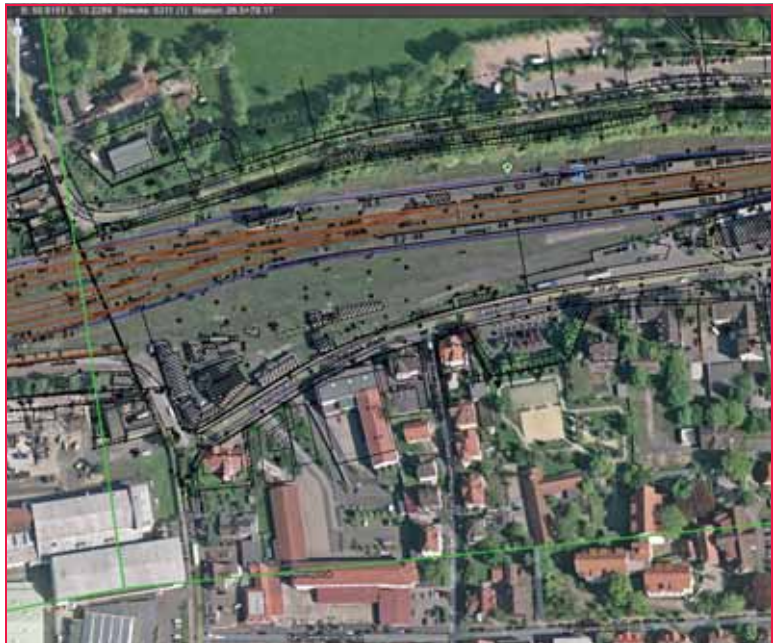
Figure 12: Position marker with information for the track and the station
