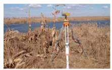
Figure 3: Base station can transmit RTK differential data and record static raw data at the same time
