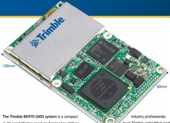
multi-constellation receiver designed to deliver centimeter accuracy to a variety of applications. The Trimble BD970 GNSS receiver supports a wide range of satellite signals, including GPS L2C and L5, GLONASS L1/L2 signals as well as Galileo GIOVE-A and GIOVE-B test satellites for signal evaluation and test purposes.
