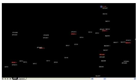
Figure 2: Control Network, a pair of GPS control points every 8 km and one bench mark every 2 km
