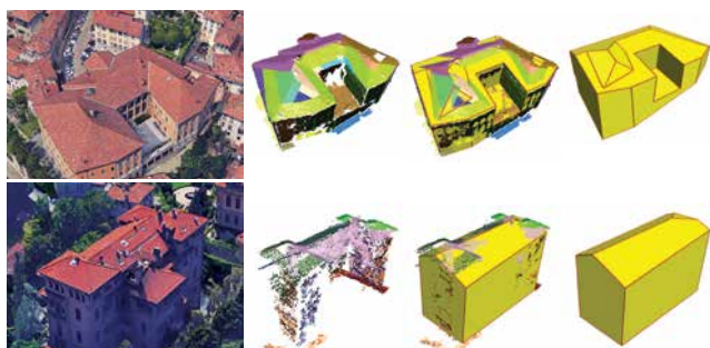
Figure 13. Examples of 3D reconstructions of different buildings from the Bergamo dataset: oblique view, planar areas of the cloud identified with RANSAC, optimized planar faces with geometric model and final 3D geometric model, respectively. Some problems are present in areas where the point density (or noise level) is not allowing a correct plane fitting
