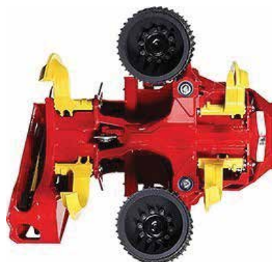
Figure 3: A harvester head with saw which cuts and delimits trees
