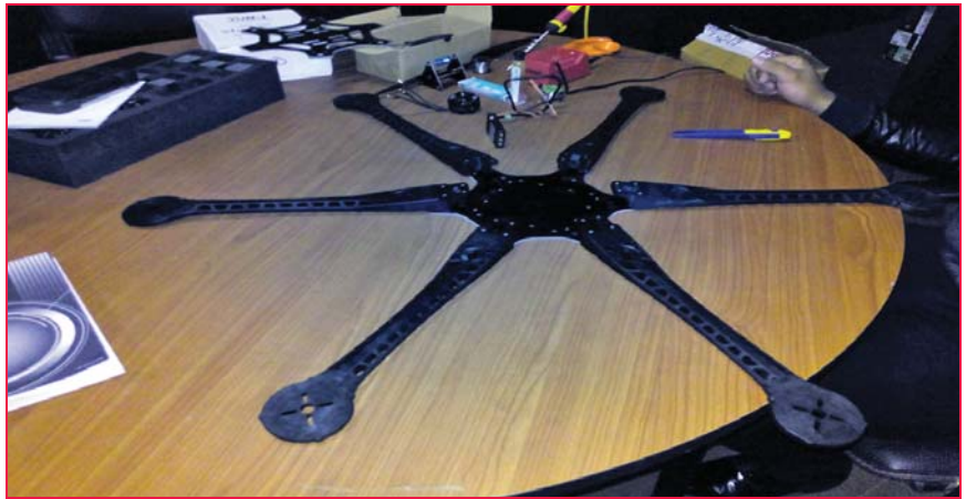
Figure 3: Hex copter frame assembled at NESAC
