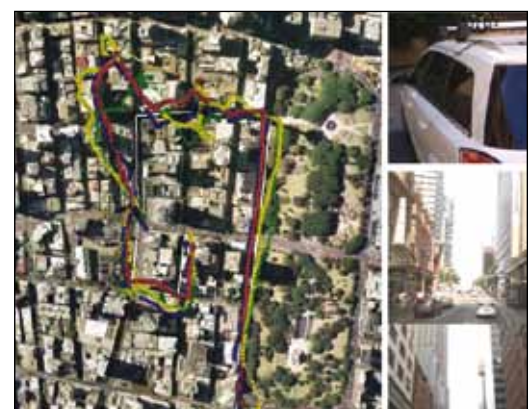
Figure 3. Kinematic test of HSGPS receivers (Navman – yellow circle; SiRF – green triangle; ublox 4 – red cross; ublox 5 – blue square; real ground track – white; start point – red star; end point – green triangle)
