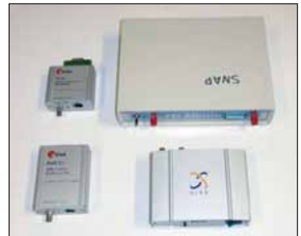
Figure 1a. HSGPS receivers used in the tests (from left to right, top to bottom: ublox LEA-4P, Navman Jupiter 32, ublox EVK-5H and SiRF GSCI-5000)
