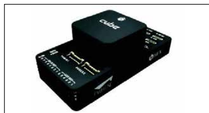
Figure 2: Pixhawk 2.1 Cube Flight Controller
