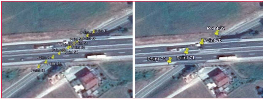
Figure 9: Positions of the peaks from the Figure B geo-located by the internal GNSS receivers of AHRS (left) and the smart phone (right).
