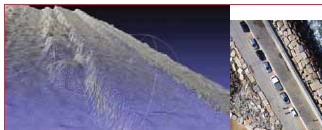
Figure 13: Meshed surface that fits the point cloud (left image): it can be seen the lower level of the superstructure with several cars on it, parked by a vertical wall. On the right an extract of one photo, taken over the same area
