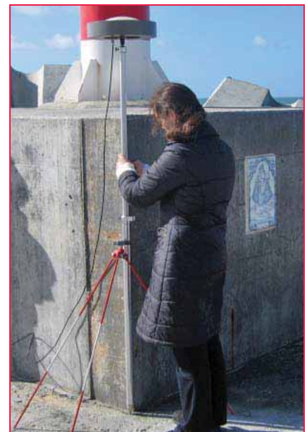
Figure 10: Coordinating a point near the lighthouse
