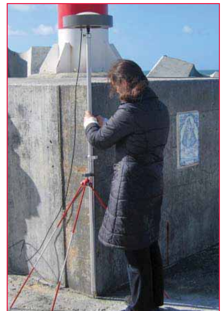
Figure 10: Coordinating a point near the lighthouse
