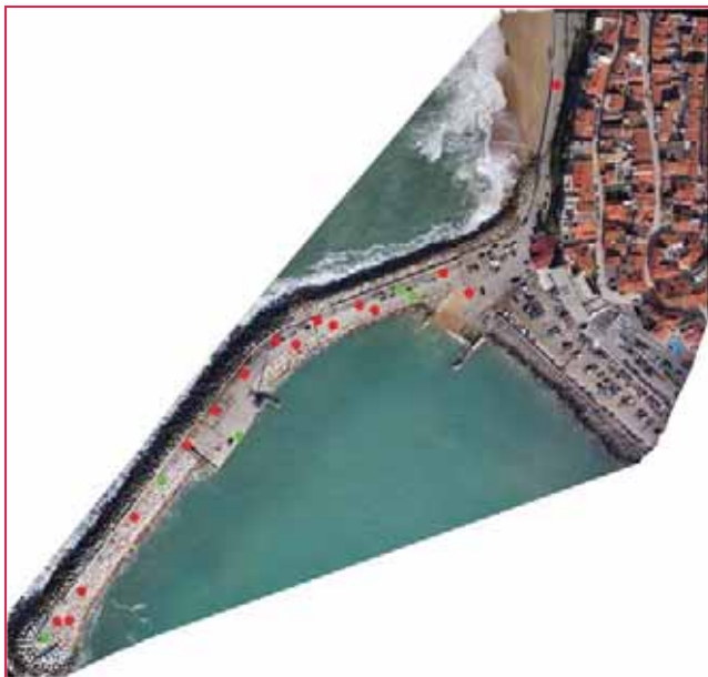
Figure 11: Orthomosaic. Location of the ground control points
