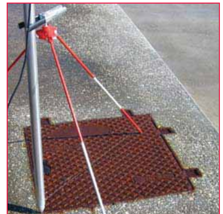
Figure 9: Southwest corner of a manhole being coordinated
