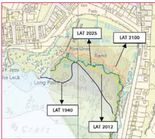
Figure 5: The shift of LAT position from 1940 to 2100 based on historical data, current survey data and 95% estimates in the high emissions scenario projected by UKCP09
