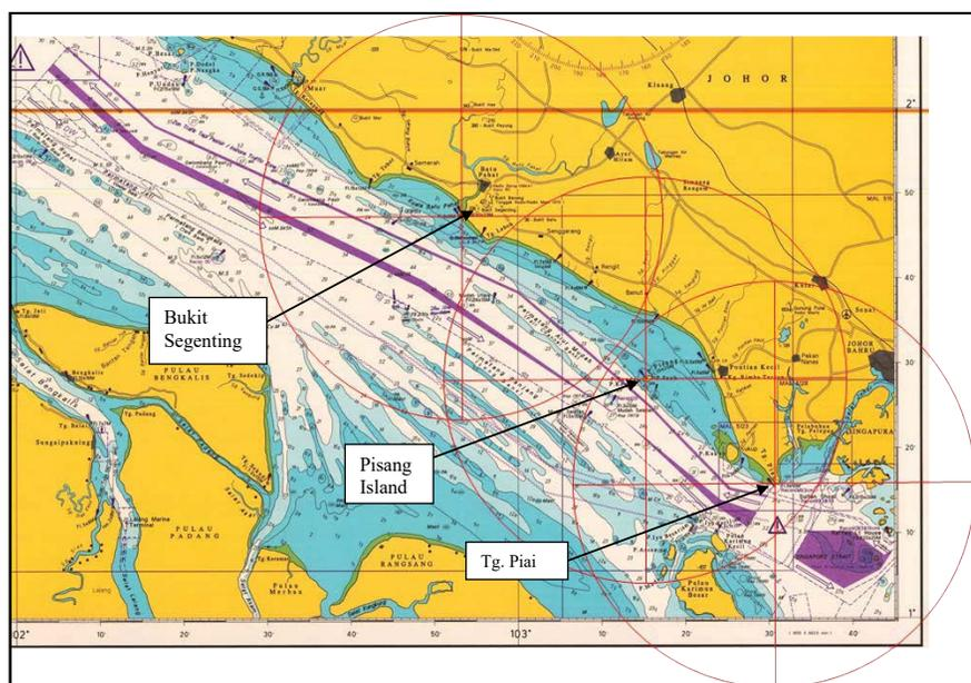
Figure 7: The proposed Pisang Island radar coverage with existing VTS radar coverage
