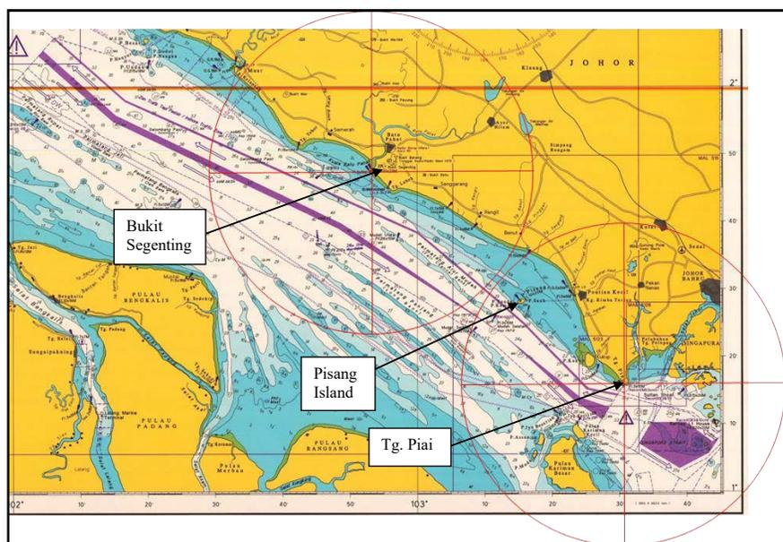
Figure 6: The existing VTS radar Coverage
