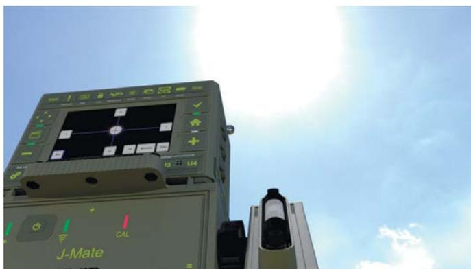
J-Mate will automatically find the Sun, and use its position to calibrate the angular encoders automatically.
