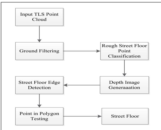
Figure 2. Flow chart of proposed method
