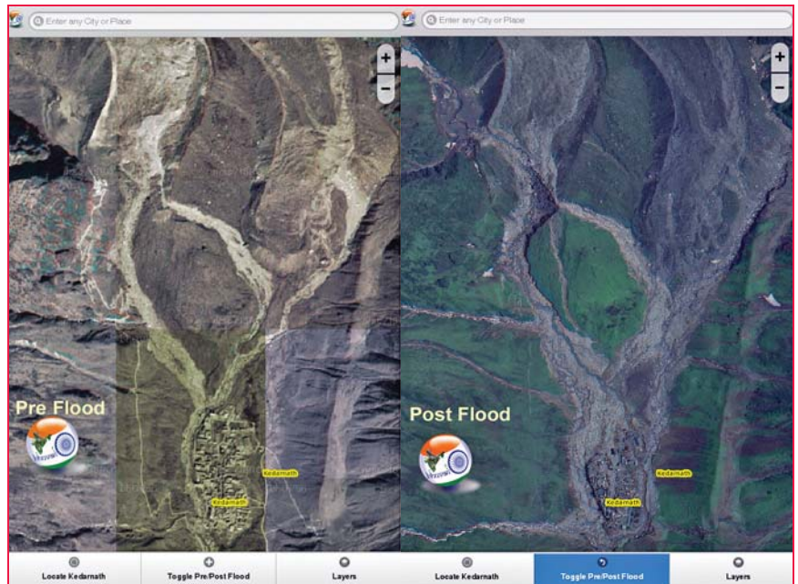
Figure 1: High resolution 1 m images generated using Cartosat 2 and LISS IV sensors, showing pre and post flood scenario around Kedarnath town. It shows the breaching of moraine at Chorabari lake, widening and creation of new channels for water and debris flow.
