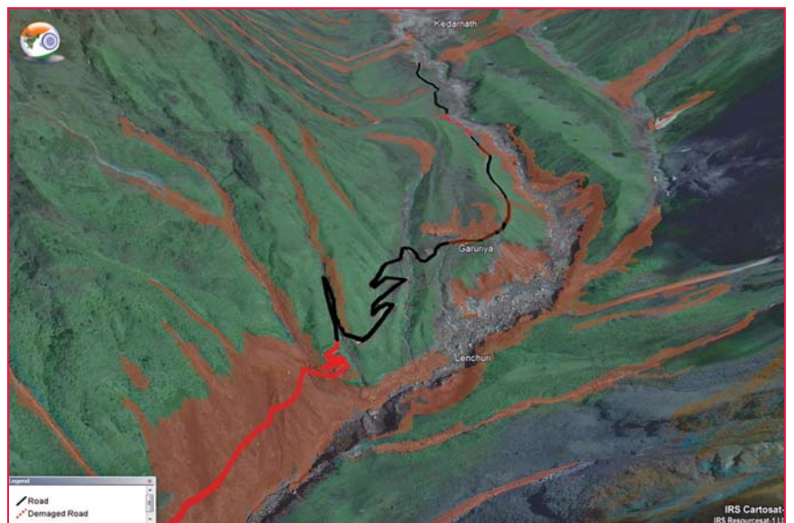
Figure 2: Post flood satellite Image showing the extent of damage caused to roads, brown color zones shows the landslides occurred during the event. Road, shown in red from Lenturi to Ghindurpani is completely damaged.
