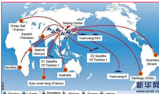
Figure 1: TT&C Network for Tiangong-1 [1]
